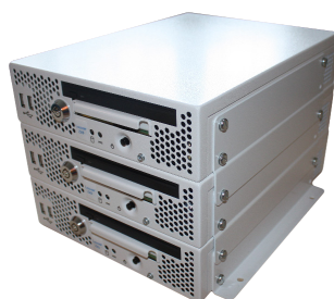
stackable modular configuration, using approved stacking brackets. (Note ZX3 illustrated)
