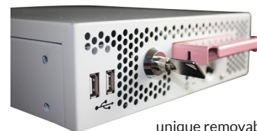
unique removable SSD drawer and locking system.
