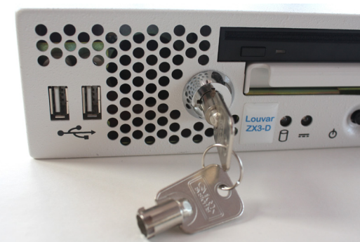
Physical security of each machine by keylock
